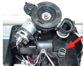
When reassembling the coffee grinder, make sure the spring is repositioned correctly (see photo).
