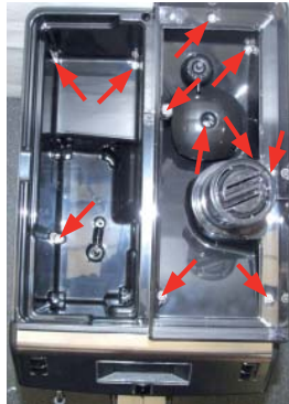
Unscrew the screws shown, raise the top cover and remove the electrical and water circuit connections.
