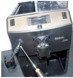
Remove the steam pipe cover as picture and unscrew the screw shown.
