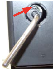
Remove the steam pipe cover as picture and unscrew the screw shown.
